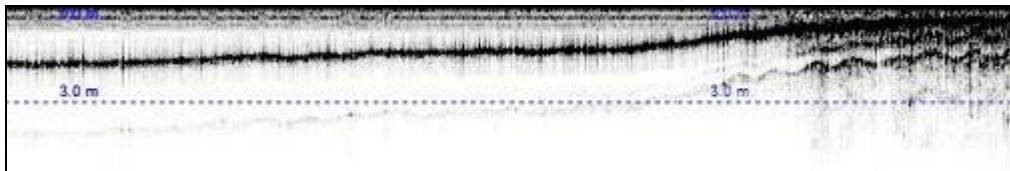
Plate 6: View of sub-bottom profile data trace, showing a perspective of the seabed's stratigraphy from close inshore (on the right side) and proceeding offshore (left side). The horizontal distance shown is approximately 70m. The vertical distance is indicated in the blue columns. The absence of any defined truncations and the absence of any hard reflectors in the section detail indicates a clean uninterrupted natural stratigraphy. The soft reflectors are associated with sand and soft silt.
